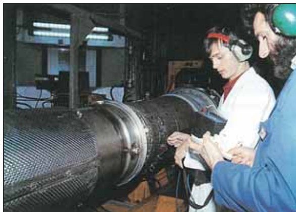
Fig. 28. Bellows for exhaust gas system of airplane engine
